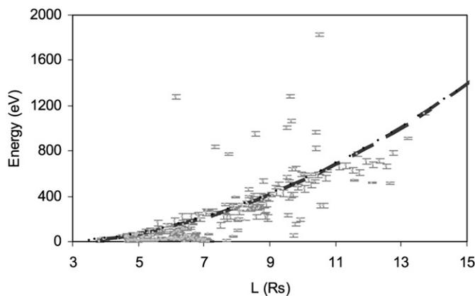
Fig. 6.  $N^+$  average energy (all detections). Average energy (eV) for each B-cycle observation as a function of L-shell for all analyzed orbits (black dots). The dotted line approximates  $N^+$  pick-up energy based on co-rotational velocity minus the orbital velocity.
