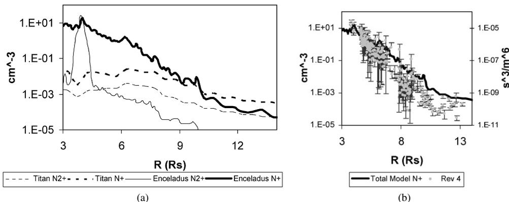
Fig. 12. Model nitrogen ion densities. Computational model nitrogen densities ( $\text{cm}^{-3}$ ): (a) vs radial distance from Saturn ( $R_s$ ) in the equatorial plane ( $Z = 0$ ) using ion lifetimes described. Thin lines represent  $\text{N}_2^+$ , thick lines for  $\text{N}^+$ , solid lines for the Enceladus nitrogen source, and dashed lines for the Titan source. Panel (b) compares the Rev 4 PSD to our total model  $\text{N}^+$  density.
