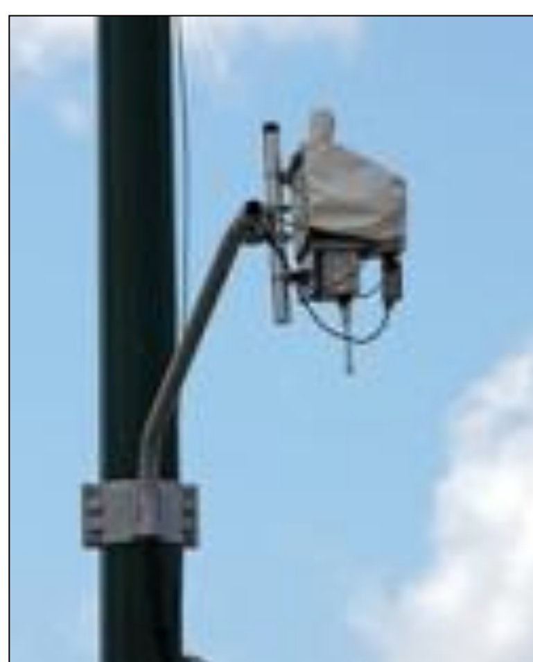
Figure 2: Road-side equipment collected vehicle information in the field
