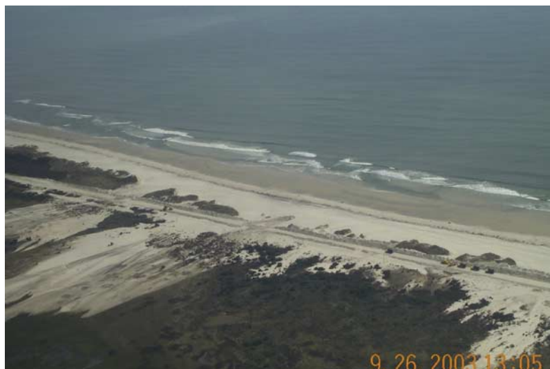
Figure 12. Overwashed sand and gaps in the dune line on Ocracoke Island, North Carolina, USA, after Hurricane Isabel in 2003. Bulldozers clearing the road and rebuilding a dune line give the scale.
