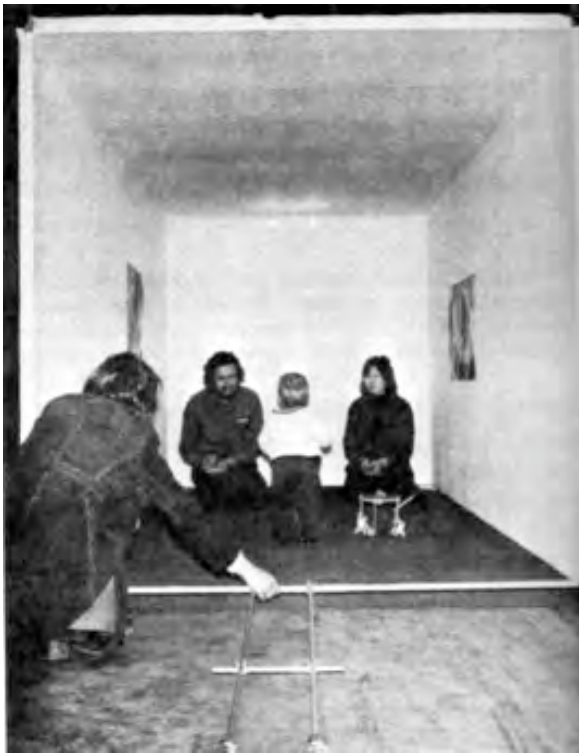
Figure 10.2: The moving room of Lee and Aronson (1974). It had three vertical sides and a ceiling, made of polystyrene foam stretched over a steel frame, but no floor. It was suspended so that it could swing noiselessly along an almost perfect horizontal path.
