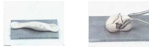
Rate dependence of viscoelastic properties in a silicone polymer (Silly Putty). Picture by Geon Corp.
