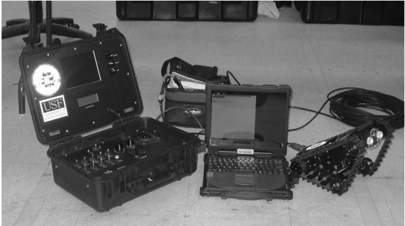
Figure 2: Full system including OCU, laptop, and robot.
