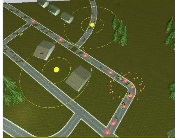
Fig. 4. The robotic swarm adapting formation to follow the truck convoy through a turn.
